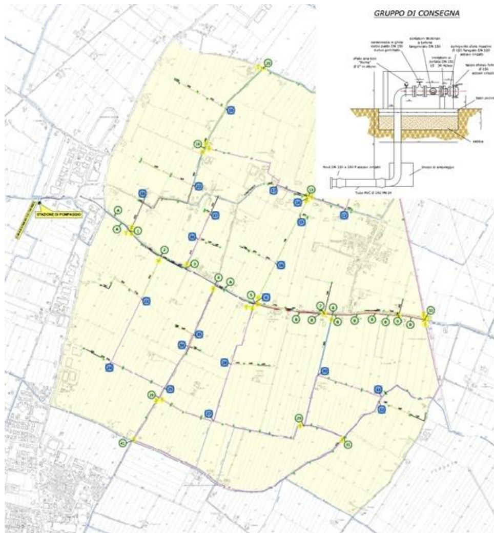
Figure 6 - Staggia Plant - irrigation pipe network
